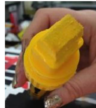
Space between nib and housing filled with paint
